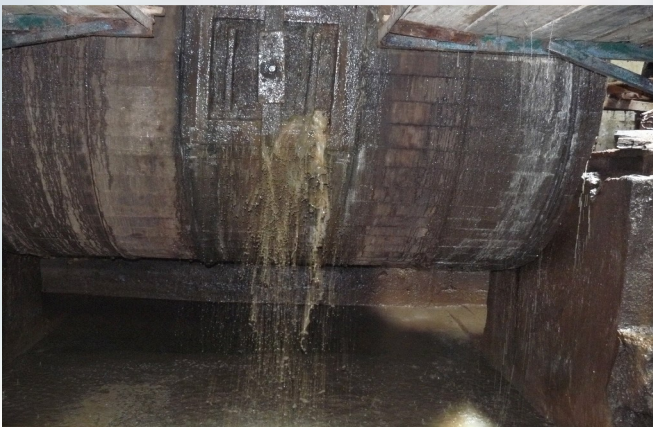
Old leaking tanning drum used before RECP
